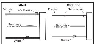
The fit of the LC200 collimator in the focuser may vary with the focuser or with a large temperature change. If it does not fit properly, adjust the nylon slot setscrews a tiny amount for a smooth fit. A little attention in this area will have a big payoff. A collimator whose axis is tilted for whatever reason cannot perform well.
